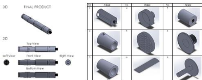
Figure 9. Final product and detail parts of prototype
