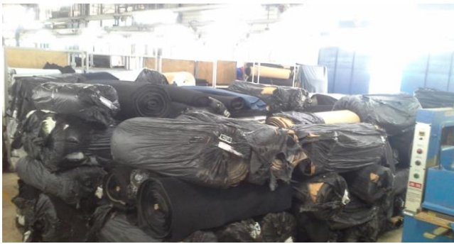
Figure 1. Material buildup in the production area
